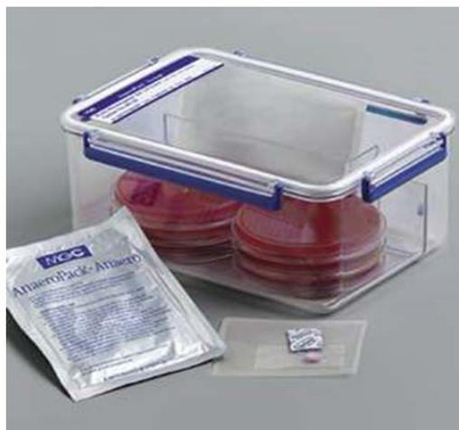
**Figure 18.** Device for incubation of transfected cells under the hypoxic condition. Low oxygen atmosphere in a hermetically closed plastic box is achieved by a combination of oxygen-absorbing and carbon dioxide-releasing organic and inorganic compounds. (figure from: <https://static.thermoscientific.com/images/F103563~wl.jpg>)
